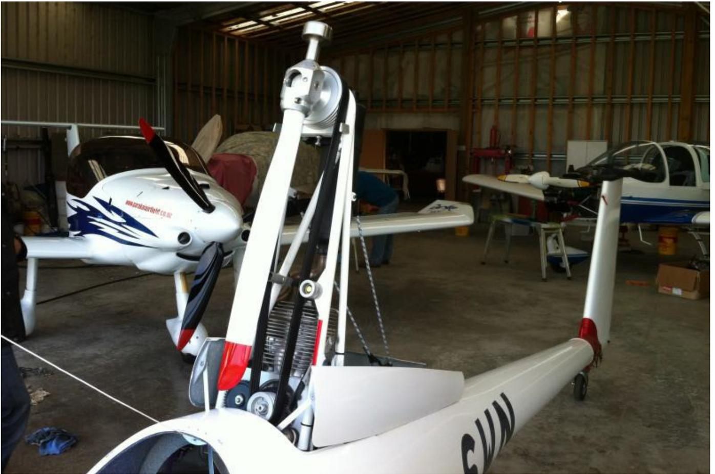
*Close up of motor, with single bladed propeller. In the background to the left is the Airport's Corporate Jet, the DynAero ZK-WIK, and to the right Tecnam ZK-JGH being serviced.*
