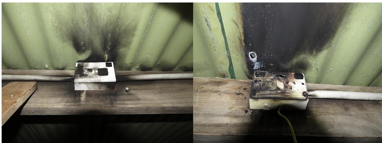
*Check out the hole blown through the corrugated Iron as the lightning exited*
