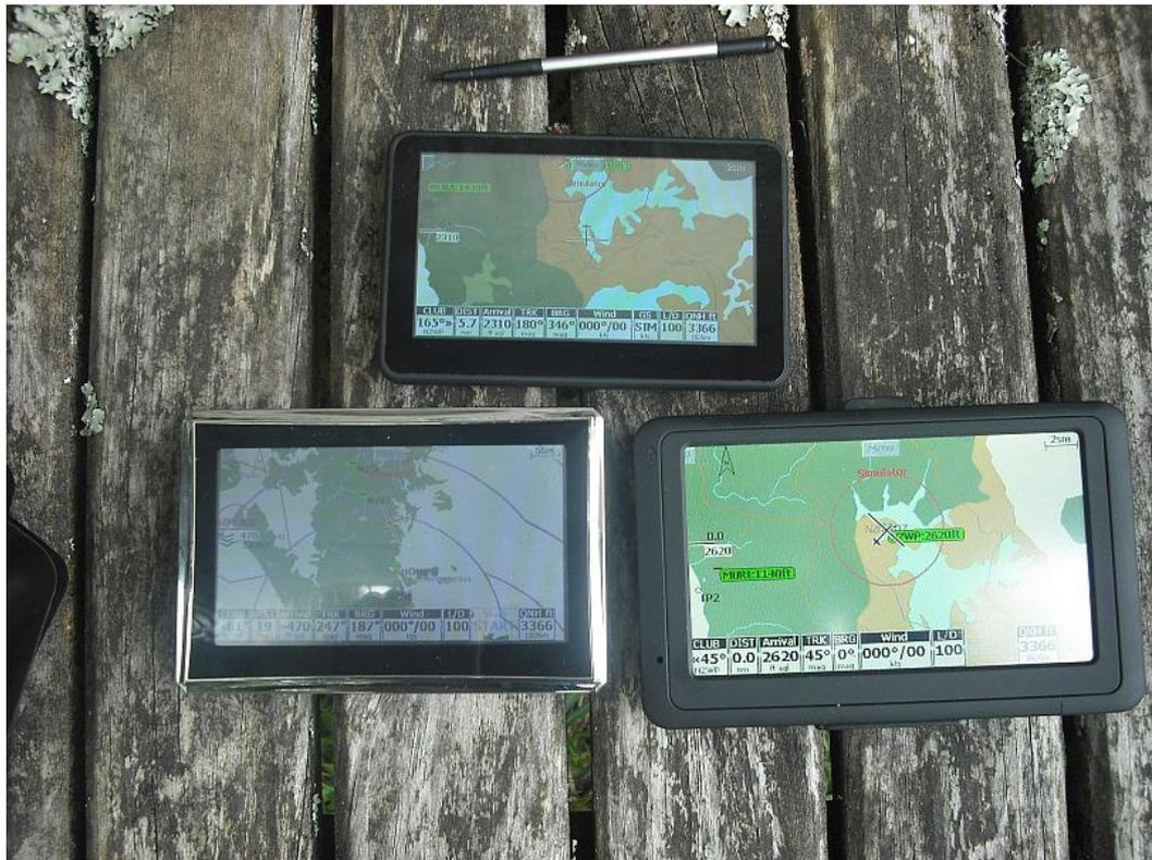
Attached please find a comparison picture showing what 800-1000 "nits of brightness" looks like compared with two generic Car GPS (supposedly sunlight readable). All three are on maximum screen brightness.
